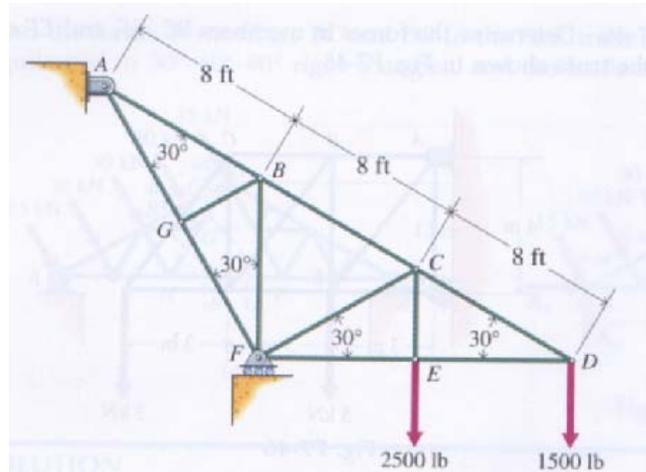
b) (15 Points) Determine the forces in members BC, CF and EF of the truss shown.
