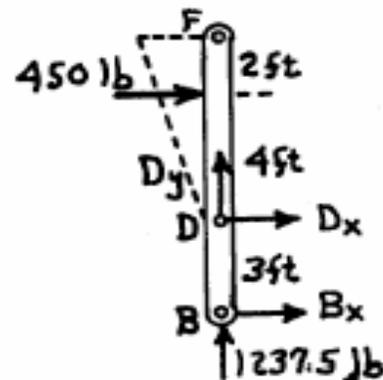
(a) From a free-body diagram of bar BDF below section aa:
